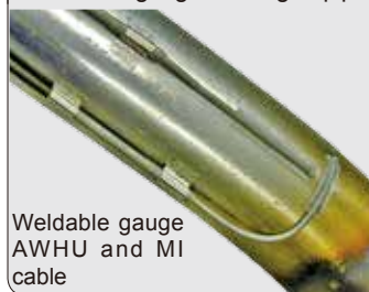
R: Bend of gauge backing or pipe
